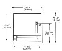
Recessed or semi-recessed towel dispenser constructed of stainless steel with exposed surfaces in satin finish. Cabinet door secured with full length piano hinge and tumbler lock. Towel dispenser operated with less than 5 lb (2.3 Kg) of force. Dispenses one standard core 8" (203 mm) or 9" (229 mm) wide x 800' (243.9 M) long paper towel roll.
