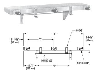
Surface-mounted utility shelf with drying rod. Fabricated of satinfinish stainless steel. Mop and broom holders of spring-activated rubber cams on plated-steel retainers.
