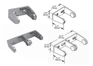
Controlled delivery. Chrome-plated, die-cast zinc. Unit features hinged arm with spring catch for filling and tension spring on fixed arm. Holds one (two) standard core roll(s) through 5" (127 mm) in diameter and 4.5" (114 mm) wide. Surface mounted.
