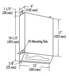
In-wall mounted towel dispenser for use behind mirror. Dispenses 800 multi-fold or 600 C-fold towels. Lock secures behind hinged dispenser lip which opens for bottom refilling.
