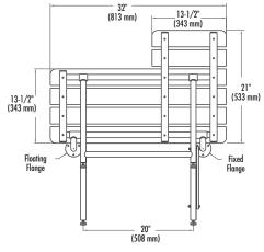
Folding bariatric shower seat with left hand configuration and barrierfree design. Frame fabricated of stainless steel tubing, 1.25" (32 mm) x 18-gauge square main frame with 1" (25 mm) x 18-gauge round cross members. Seat of 0.5" (13 mm) thick solid phenolic with white matte melamine finish. When properly installed, designed to support at least 900 lb (408.2 Kg).
