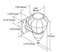
Liquid soap dispenser features chrome-plated bracket, translucent polyethylene globe and push-up-type valve with corrosion-resistant components and vacuum-flow control. Holds 16 oz (473 ml) liquid soap. Swivels for filling
