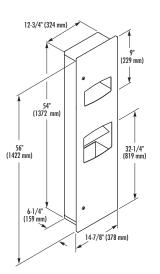
Convenient, space-saving 3-in-1 towel dispenser, hand dryer and waste receptacle. Constructed of architectural satin finish stainless steel. Recessed towel dispenser holds 710 single-fold, 500 multi-fold or 370 C-fold paper towels. Waste receptacle has 4.37 gal (16.5 L) capacity. Hand dryer has sensor activation with universal voltage.
