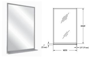
Channel-framed mirror with shelf. 0.75" x 0.75" x .4375" (19 mm x 19 mm x 11 mm) frame of stainless steel with bright annealed finish. Neatly mitered corners. 0.25" (6 mm) thick glass. 5.5" (140 mm) W satin finish stainless steel shelf welded to frame. Wall hanger of 18-gauge steel provides vandal- and theft-resistant mounting. Galvanized steel back plate with shock-absorbing, waterproof filler.
