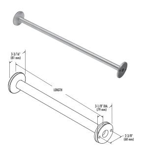
Heavy-duty shower curtain rod with concealed mounting. Fabricated of satin-finish stainless steel; 1.25" (32 mm) O.D. Flanges 3.1875" (81 mm) O.D. Escutcheons snap over flanges to provide concealed mounting. For lengths 72" (1829 mm) and greater, model 9522 (ceiling support) is required. Must specify distance from ceiling.
