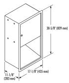
Constructed of architectural satin finish stainless steel. Dispenses singlefold, 800 multi-fold or 500 C-fold towels.
