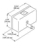
Surface-mounted, stainless steel with architectural satin finish. Locked cover removes for filling. Holds 44 oz (1301 ml) liquid soap. Push-intype valve delivers measured amount of liquid soap.
