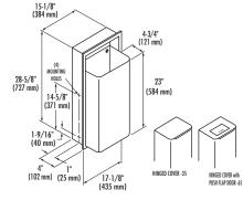
Recessed, 12-gallon, removable, stainless steel waste receptacle. Secured to cabinet with tumbler lock. Heavy-duty, reusable, 12 gal (45.4 L) liner available as an accessory. Order separately using part number P11-004.
