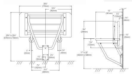
Folding, Bradmar'' solid plastic shower seat. Stainless steel tubing with stainless steel wall bracket and piano hinges. Seat of 1" (25 mm) thick high-density polyethylene. All exposed edges are machined smooth. Square configuration. Folds to vertical position when not in use. Designed to support up to 400 lb (181.4 Kg) static load.
