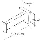
Surface-mounted stainless steel clothes hook. Exposed mounting.
