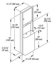
Constructed of architectural satin finish stainless steel. Dispenses 475 multi-fold or 350 C-fold towels. Waste receptacle has 2 gal (7.6 L), removable, stainless steel insert.
